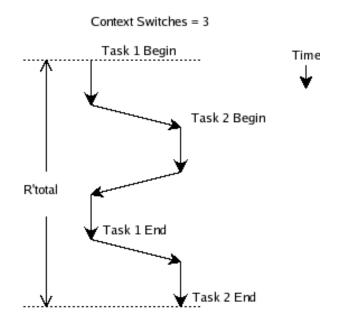
For n context switches with direct overhead C, the total indirect overhead  $I = R'_{total} - (R_{total} - C) - n \times C$
