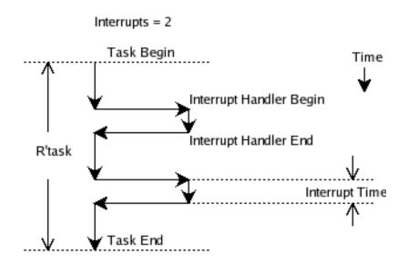
If the direct overhead in servicing the timer interrupt is D, the total indirect overhead is  $I = R_{task}^{'} - R_{task} - n \times D$
